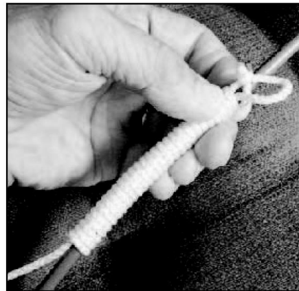
Figure 4 — When done, you will have about 3.5 inches of rope wrapped around the coax.
