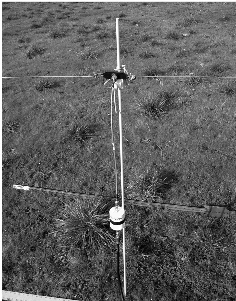
Figure 2 — Center connector, common mode choke and feed point support.
