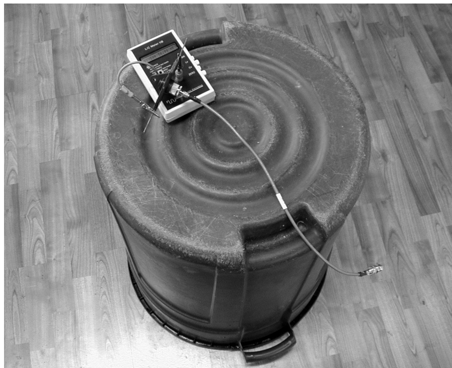
Figure 3 — Shunt capacitance measurement of the center fitting.
