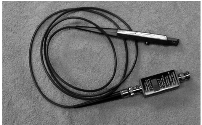
Figure 34 — Scope probe used for current pickup.
