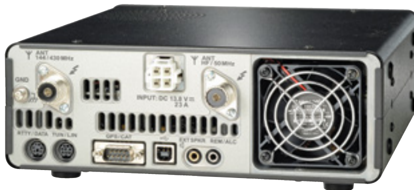
Figure 1 — The FT-991’s rear panel, showing available connections.
