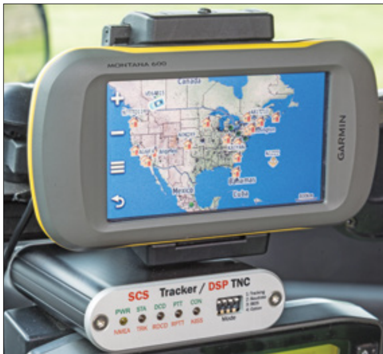
Figure 19 — The SCS Tracker/DSP TNC in the author's mobile station, with its companion Garmin Montana GPS receiver. The screen displays icons showing the locations of stations on the network.
