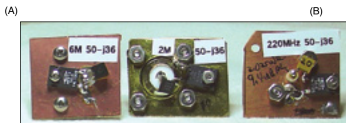
Figure 14 — At A, the 7.5 \Omega , 400 \Omega and complex loads for 50, 146, and 222 MHz. At B, the component side of the three complex loads
