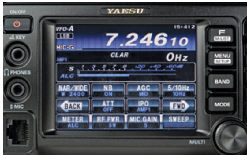
Figure 5 — The FT-991's display is crisp and conveys a lot of information about current operating parameters. The three rows of rectangular labels at the bottom of the screen are touch-sensitive buttons. The buttons change as different modes, features, or menus are selected.
