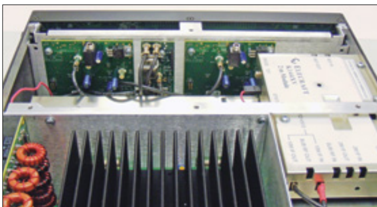
Figure 9 — Inside view from the rear of the author's dual-receiver 100 W K3 with new synthesizer boards installed.
