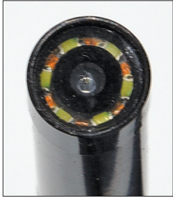
Figure 5 — The business end of the Depstech endoscope features a miniature video camera and six bright LED lights.
