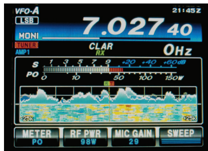
Figure 1 — The FT-991A's colorful touch-screen features a new real-time spectrum display. This view shows both a traditional spectrum scope (panadapter) and a waterfall display.
