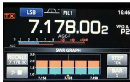
Figure 7 — The SWR graphing function offers a visual indication of antenna system SWR over an adjustable frequency range.
