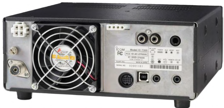
Figure 1 — The IC-7300’s rear panel has connections for a CW paddle for the internal keyer or external key/keyer; an external speaker; ALC and TR switching for an amplifier; remote control via the optional RS-BA1 software or an Icom CI-V device; a USB port for radio control and digital mode operation; an ACC socket for connecting a TNC or PC for digital modes, and a jack for connection to any of Icom’s accessory antenna tuners or tuned antennas.
