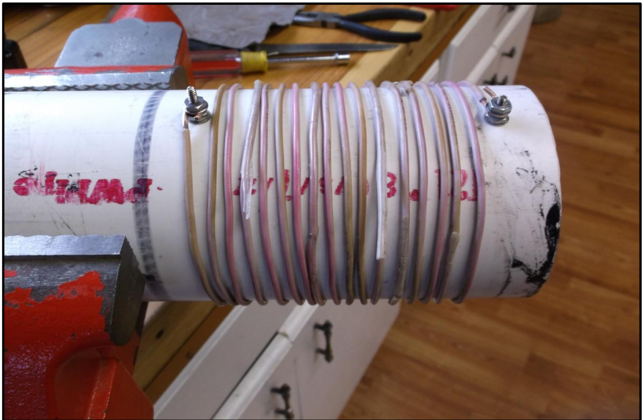
Figure 2 - Old radial wire wound into an inductor.
