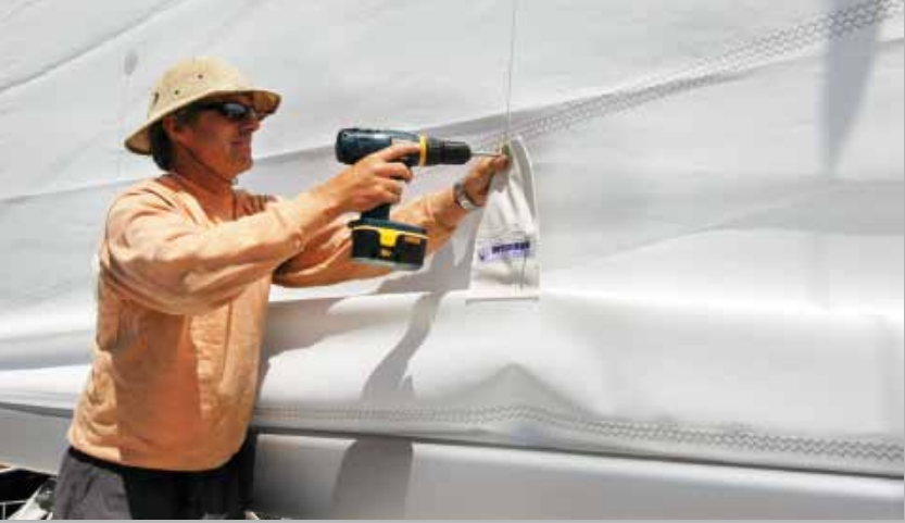
An electric screwdriver is used to attach clips that secure the Dutchman's line storage bags. (Photo by Ralph Naranjo)
