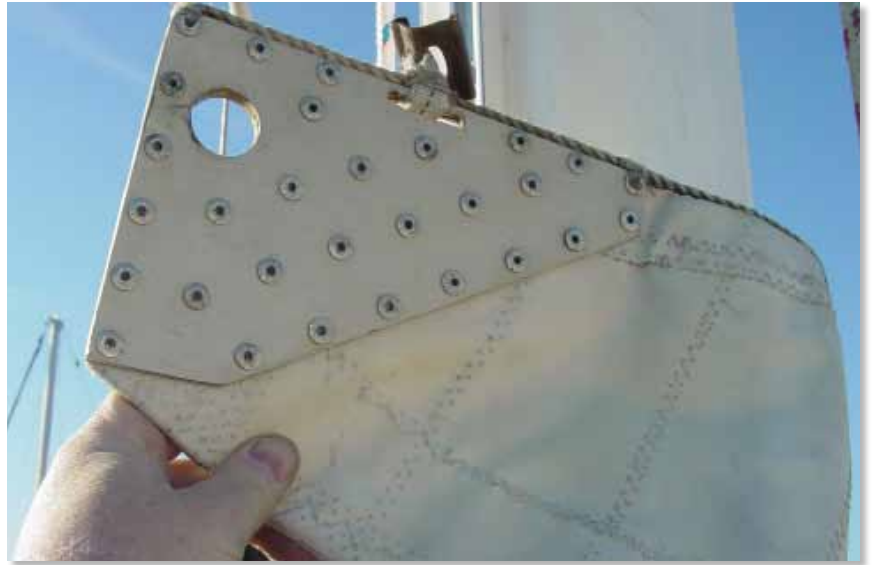
The original mainsail left plenty of room for improvement. The external slides (above), though reliable, put a lot of friction on the luff. The stack height (left) was hard to manage. (Photos by Frank Lanier)
