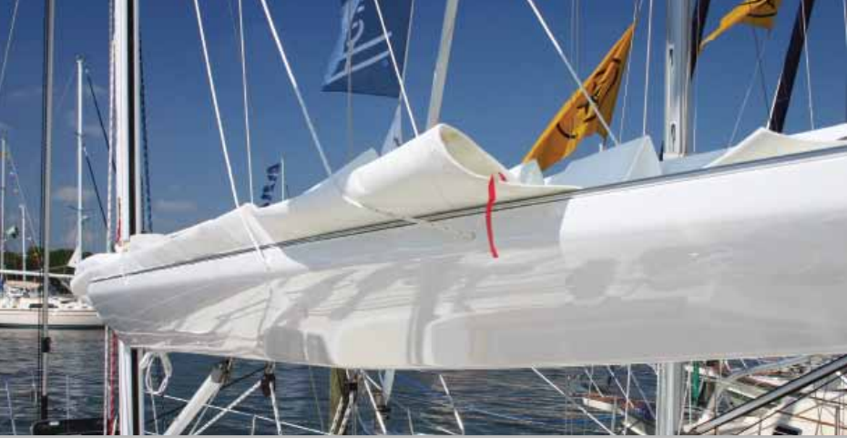
Tartan Yachts' carbon-fiber Stow-Boom neatly catches a fully battened sail. .....
