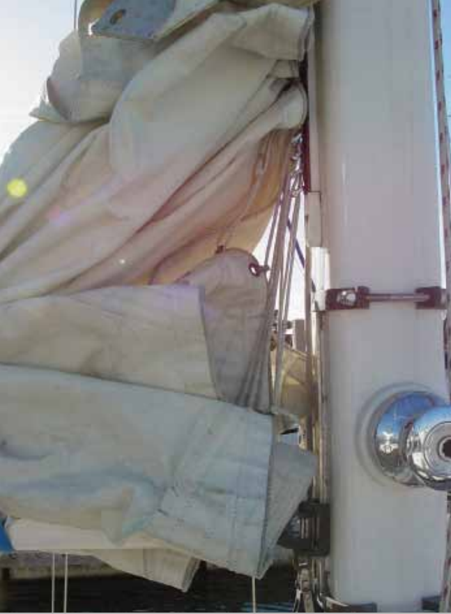
The original mainsail left plenty of room for improvement. The external slides (above), though reliable, put a lot of friction on the luff. The stack height (left) was hard to manage. (Photos by Frank Lanier)
