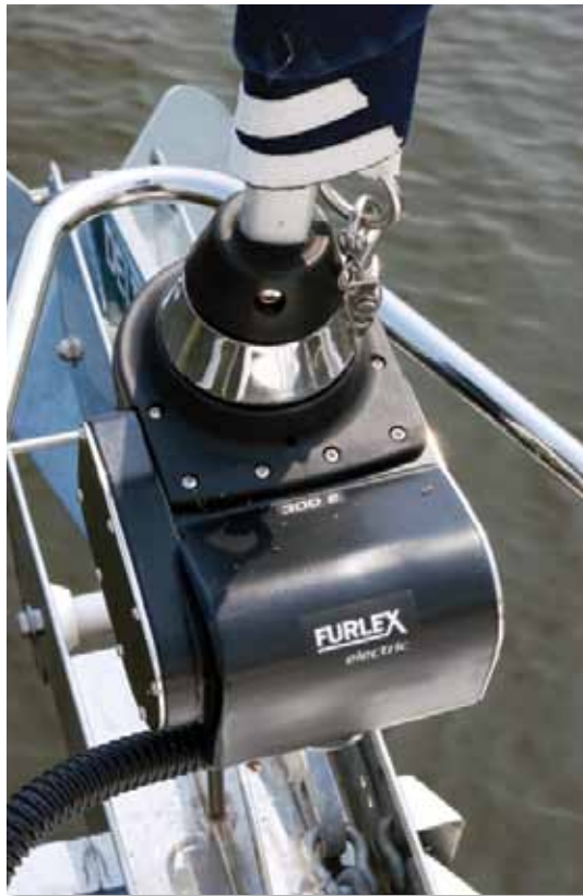
The Furlex Electric can turn an existing or new manual Furlex into a power furler. .....
