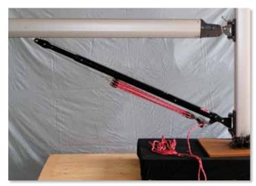
The Forespar Yacht Rod is one of the easiest to adjust vertically after installation.
