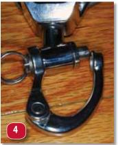
1.)Testers liked the design execution of the Antal 9060's side-opening block. 2) The one-handed, push-button Harken was testers' favorite. 3.) The line must be bent slightly to fit into the side-opening Garhauer. 4.) The trunnion-type snap shackle on the Harken block uses the locking pin as a pivot point, allowing a full range of motion.
