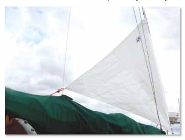
the FinDelta Anchoring Sail from Banner Bay Marine, which uses three panels instead of the traditional single panel. While the traditional riding sail has served sailors well for centuries, this new design intrigued our testers, and a head-to head-comparison was launched.
