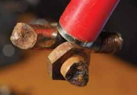
under-load failure seen in the older products we inspected provided insight into potential failure modes.
