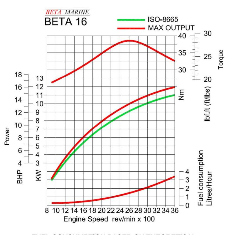
FUEL CONSUMPTION BASED ON THEORETICAL PROPELLER LOADING - MATCHED AT FULL SPEED.
