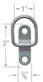
3/16" Hinged Pad Eye Safe Working Load: 400 lbs
