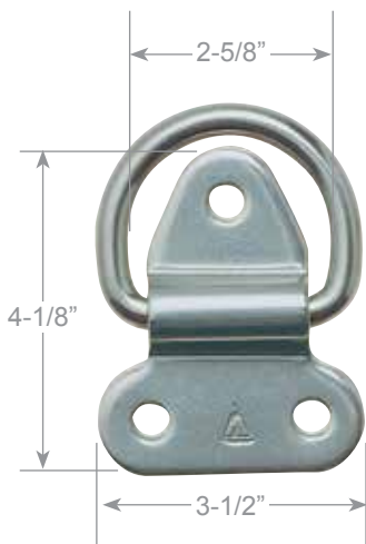
1/2" Hinged Pad Eye Safe Working Load: 3500 lbs
