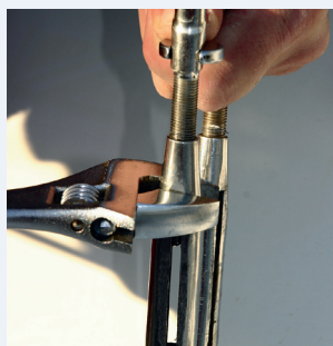
Using ordinary hand-tools on the bottlescrews, it's hard to over-tension the rigging
