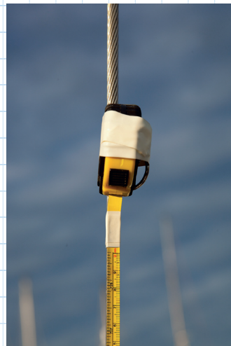
To measure the stretch, extend a tape measure (or ideally a folding rule) to 2,000mm and mark this distance up the wire...
