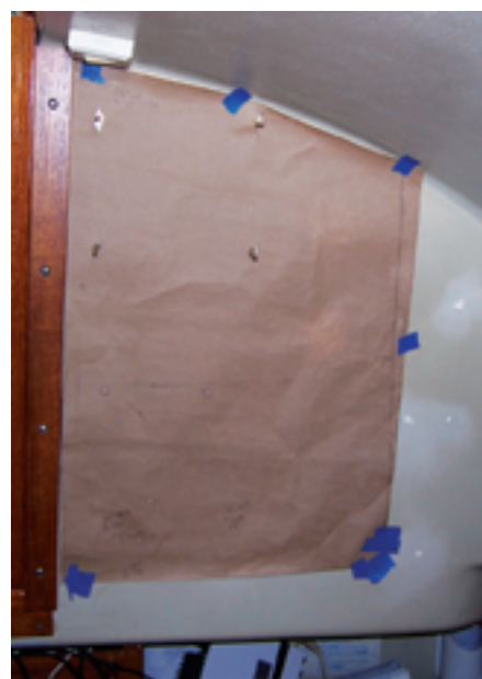
This view of the backs of electronic navigation devices detracted from the cabin's ambiance. Tony's plan for concealing them began with a piece of kraft paper on which he marked critical dimensions and the locations of the instruments and their wires.
