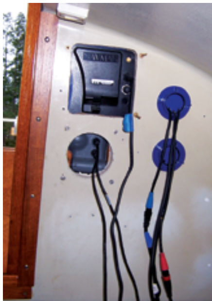
This view of the backs of electronic navigation devices detracted from the cabin's ambiance. Tony's plan for concealing them began with a piece of kraft paper on which he marked critical dimensions and the locations of the instruments and their wires.
