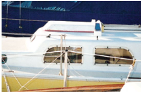
From every angle, the sea hood blends into the boat's original lines. Its crown follows that of the cabintop, far left, and its forward face follows the slope of the step in the cabin, near left.
