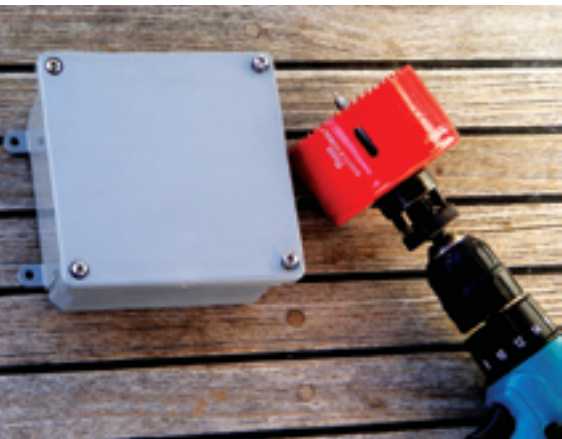
Instead of taking the big hole saw to his cockpit coaming, he took it to the cover of the junction box.
