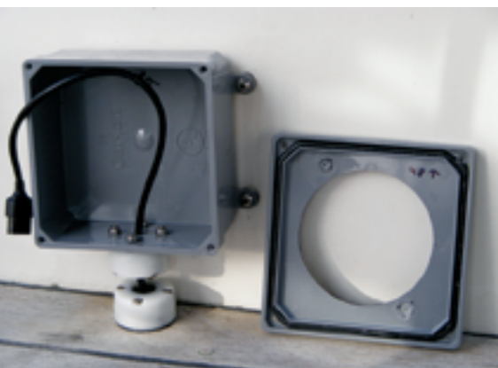
After leading the cable through two Cable Clams, he attached the box to the cockpit side.
