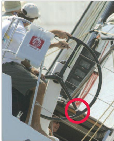
When the piece of white tape on this spoke (red circle) is at the top of the wheel, the rudder is centered. This boat currently has about 'one spoke' of windward helm. An obvious mark like this makes it easy for the entire crew to see how much helm the boat has at any particular moment.
